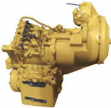
**Five-Speed Transmission.** The field proven Cat power shift countershaft transmission easily matches engine power to the load size and ground conditions. Electronic control makes fingertip controls possible, reducing operator fatigue and improving comfort.
