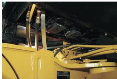
**Hitch Hoses.** The pilot hoses, pressure line and load sense lines have all been routed above the hitch, and been bulk-headed for easy hose replacement and fast service.
