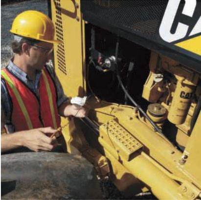
**Engine Enclosures.** Large, hinged engine enclosure doors make regular maintenance as easy and fast as possible. Easy access to daily service points increases the likelihood that maintenance will be done, and increases machine service life. In addition, less maintenance time means more working time and greater productivity.
